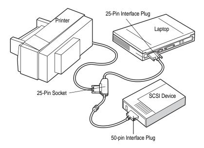
Figure 1. Typical Installation
